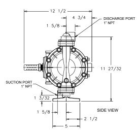
BOTH SUCTION AND DISCHARGE PORTS ARE AVAILABLE WITH 1" BSPT TAPERED THREADS (41-818823 STAINLESS STEEL ONLY)
