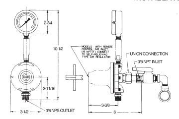
Installation is simplified by the use of a swivel nut inlet connection (see photo). This is standard on all models; it eliminates the cost of a union, and provides a quick and convenient method to easily remove the unit from the line.
