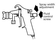
**Spray width adjustment:** Turn clockwise for round, counterclockwise for fan.
